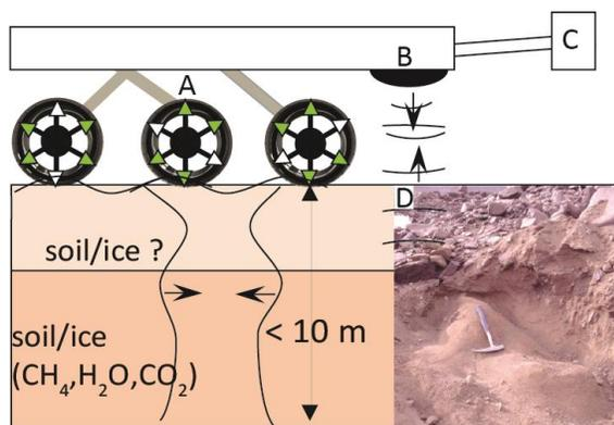
**Figure 1.** A. Alternating seismic sensors (green) and sources (white) receive and send seismic waves. B. Ground-penetrating radar transceiver detects pore-space substituted with ice. C. A long-arm gamma-neutron spectrometer. Sensor collects nuclear spectra away from influence of rover. D. As a specific example for Mars, the Antarctic Dry Valleys analog [2] implies a potentially complex soil-ice mixture for Mars that requires an integrated suite of geophysical and geochemical tools.
