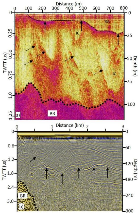
**Figure 2.** a) 100 MHz GPR Profile along the flank of Mount Waesche showing re-advanced ice (RA) over debris (dashed black line, arrows), dipping debris bands within deeper ice, ice cored features (IC), and bedrock (BR). b) 5 MHz GPR profile showing unconformity reaching 120 m depth and surface conformable stratigraphy distal to Mount Waesche.
