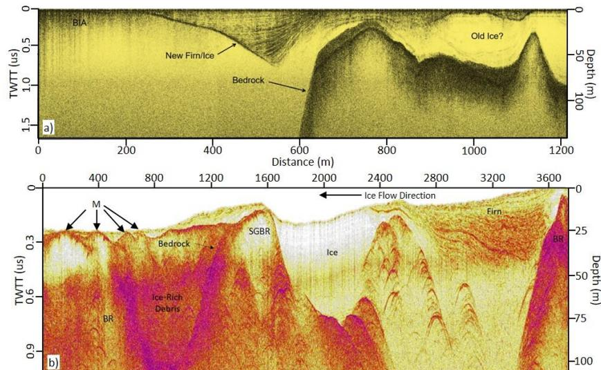
**Figure 3.** a) 100 MHz GPR profile from Pensacola Mountains, showing new firm deposited over blue ice, a bedrock rise, and likely old stagnated ice due to topographic blocking of flow. The profile is oriented approximately parallel to ice flow from Thomas Hills (right) towards Foundation Ice Stream (left). b) 100 MHz profile from Ohio Range showing firm over blue ice that is stagnated against a sub-glacial bedrock rise (SGBR) and a series of ice cored moraines (M) over ice-rich debris.
