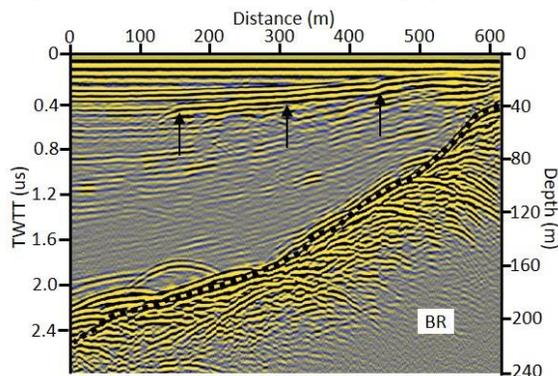
**Figure 1.** 10 MHz Ice Radar profile from Mount Murphy, Thwaites Glacier, showing shallow unconformity near 30 m depth (black arrows), and bedrock (BR) at and below approximate dashed line.
