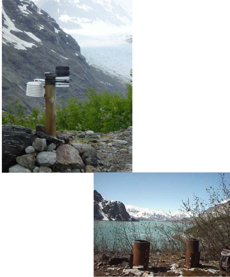
Figure 2. Typical climate sites. Upper left photo shows white solar radiation shield housing temperature sensors and a tipping bucket rain gauge installed on 1-meter tall post at Muir Glacier. Photo on lower right shows the tipping bucket and electronic rain gauges in steel housings as mounted on the ground at the Riggs site. A post can only be used where animals are unlikely to damage rain gauges, but preferred wherever possible to reduce snow cover effects on winter season data.
