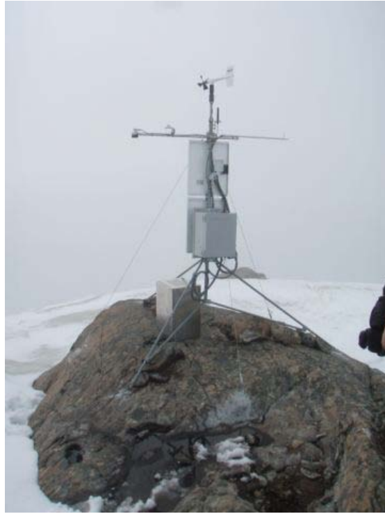
Figure 3. Climate station for high altitude sites shown at Columbia Glacier (photo: D. Finnegan). The Iridium satellite antenna is the ~6 in. black rod on the right side of the tower below the wind sensor. The long arm extending to left holds a snow depth sensor. Data are stored within data logger in the gray box on the mast and may be transmitted at various rates from minutes to hours. Two-way communication allows commands such as changing frequency of data collection and transmission from office computers.
