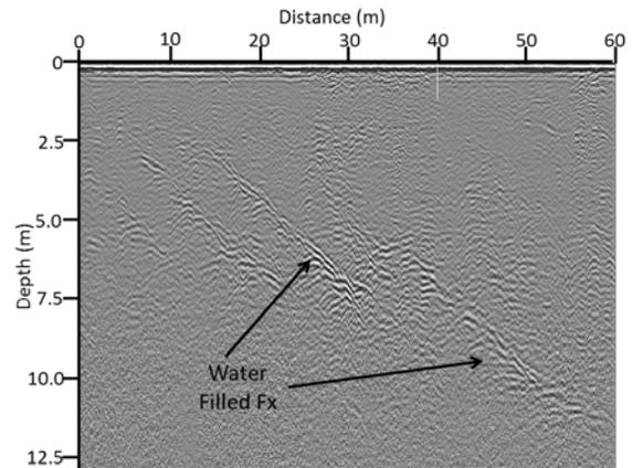
Figure 2: 400 MHz GPR profile showing parallel water filled bedrock fractures (Fx) on Mount Adams, NH.
