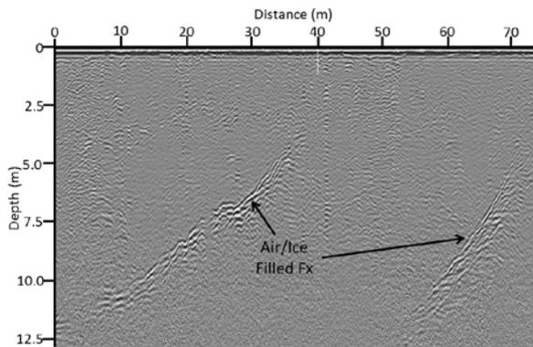
Figure 1: 400 MHz GPR profile showing parallel bedrock fractures (Fx) within a zone of Mount Adams, NH.
