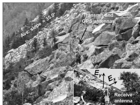
Fig. 1. The talus slope of angular boulders. Transmit and GPS antennas are carried along a linear across-slope transect. Insert shows receiver Yagi antenna and polarizations
