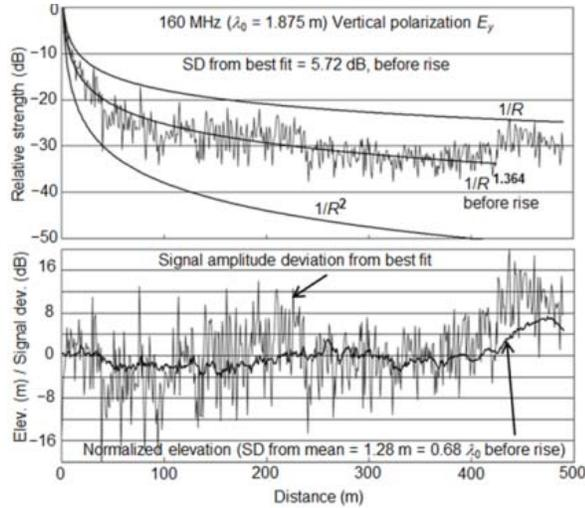
Fig. 2. Amplitude and elevation for the along-slope vertical polarization transect.
