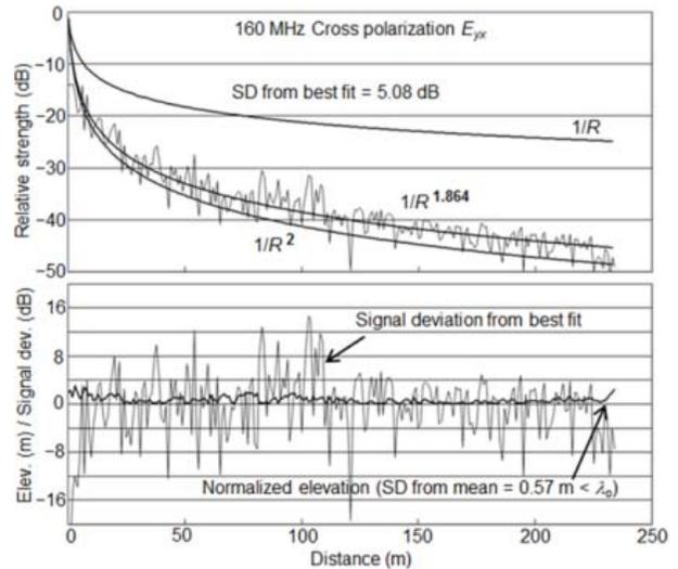
Fig. 5. Amplitude and elevation for the down-slope cross polarization transect.
