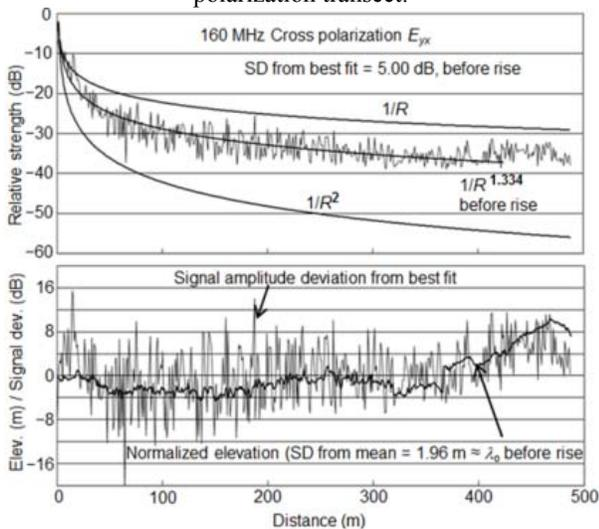
Fig. 3. Amplitude and elevation for the along-slope cross polarization transect.
