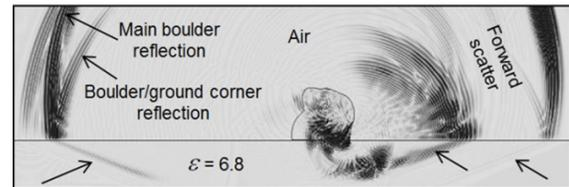
Fig. 6. 2-D simulation of pulse encountering a  $7 \lambda_0$  size dielectric ( $\epsilon = 6.8$ ) boulder. Arrows indicate forward and back head waves. Note strong forward boulder scatter.
