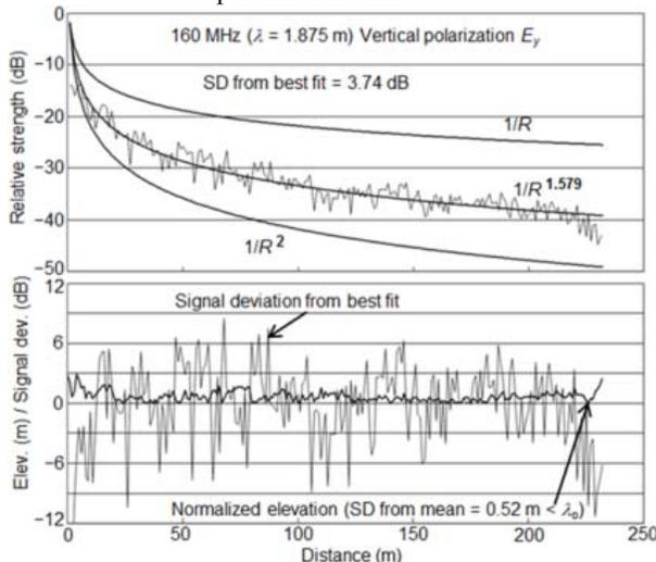
Fig. 4. Amplitude and elevation for the down-slope vertical polarization transect.
